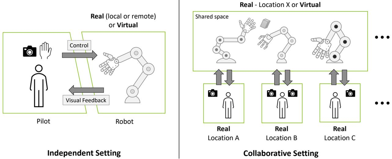
Fig. 2: Paradigms of vision-based teleoperation systems in *independent* and *collaborative* settings. The system should support any arm-hand models, existed in either virtual or the real world, can operate with flexible camera configurations, provide visual feedback for both local or remote presence, and support multiple robots piloted in a shared space.
