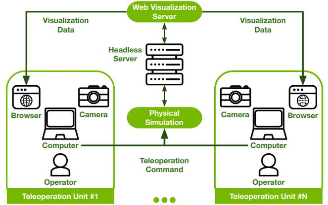
Fig. 6: **Collaborative Teleoperation System.** Our system can be extended to collaborative manipulation tasks even when operators are not in the same physical location. Each operator can use a local computer with camera to detect the hand pose and send the detection results to a central server. Meanwhile, they can use the web browser to visualize the current simulation environment, including the robot controlled by other operators.
