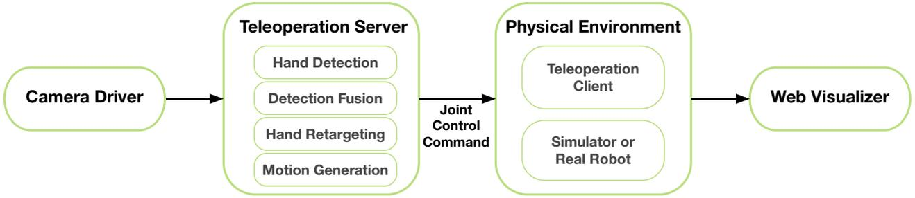
Fig. 3: **System Architecture.** AnyTeleop is composed of four components: (i) camera driver, which captures the human hand pose in RGB or RGB-D format; (ii) teleoperation server, the core component in our system, which performs hand pose detection and converts detection results to robot control commands; (iii) teleoperated robot, which is either a real robot or a simulated robot in a virtual environment; (iv) web visualizer, which enables remote visualization across the internet.
