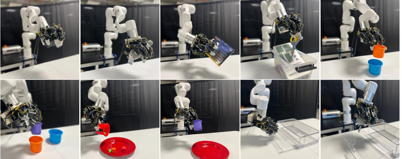
Fig. 4: **Real Robot Teleoperation Tasks.** We replicate the ten manipulation tasks proposed in Sivakumar *et al.* [54] using same or similar objects. Top row, left to right: Pickup Box Object, Pickup Fabric Toy, Box Rotation, Scissor Pickup, Cup Stack. Bottom row, left to right: Two Cup Stacking, Pouring Cubes onto Plate, Cup Into Plate, Open Drawer and Open Drawer and Pickup Cup.
